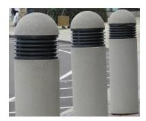
Using LED technology as the lighting source in the bollards would reduce electricity use by approximately 50% and extend longevity by approximately 4 times to 50,000 hours; this means no maintenance for approximately ten years. A total of sixteen bollards were counted on site.
